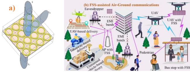
Figure 2.- a) Schematic representation of a Frequency Surface Selective with ring elements. 'S' is the incident wave, 'S r ' is the reflected wave, and 'S t ' is the transmitted wave. b) Illustration of FSS-assisted future 6G networks.[25]
